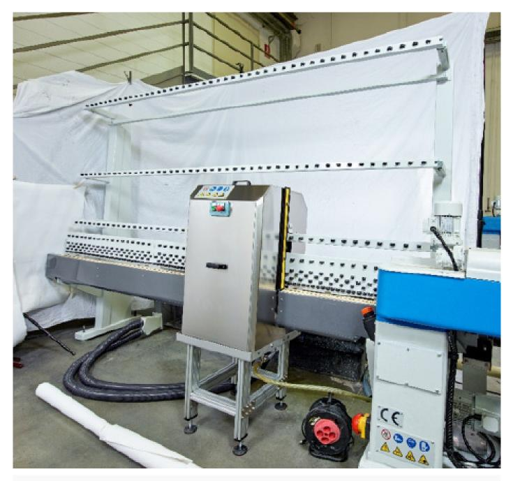
washing machine on outlet conveyor LV 322-40.
