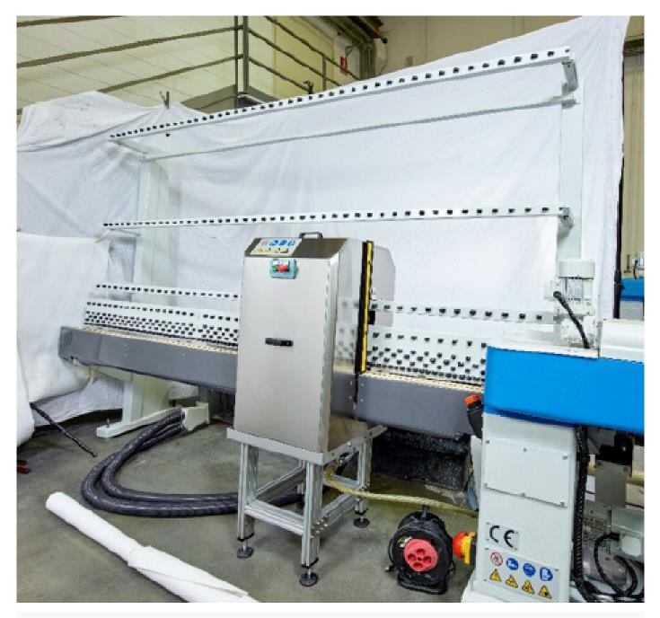
washing machine on outlet conveyor LV 322-40.
