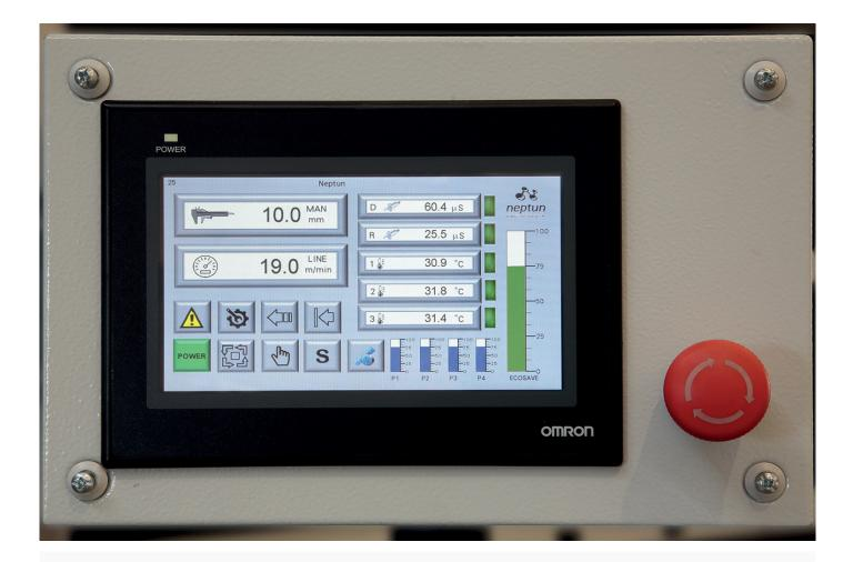
At a preset time set on the control panel, the NC activates the automatic emptying of the tanks, at the end of which they are refilled so as to have new water at the beginning of the shift. The function can be set for each day of the week
