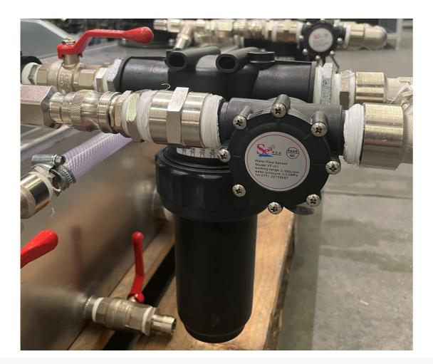
Flow switches to check the filter cleaning status
