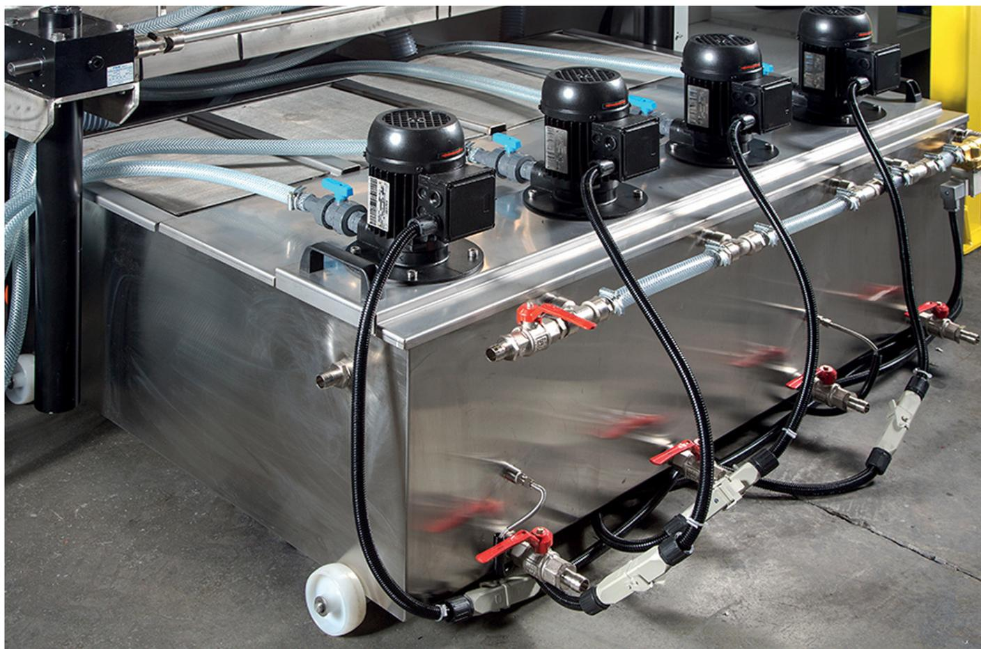
Possibility of heating the water and maintaining the temperature up to 60 °, with resistances, thermostats and resistance protection sensors in the event of a drop in the water level. Extremely compact removable stainless steel tank for minimum bulk and easy maintenance.
