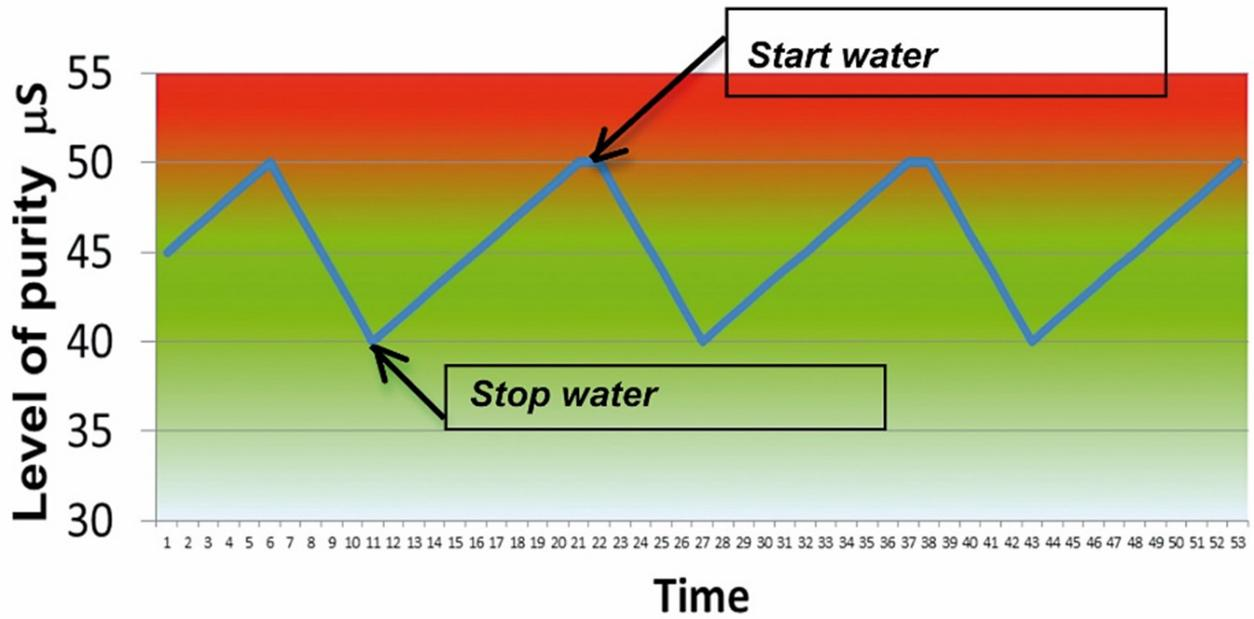
Water circuits that can be configured according to the application, with inlet and outlet filters, pumps and dedicated tank sections. Water quality control and management system, which automatically feeds clean water according to the required level of purity
