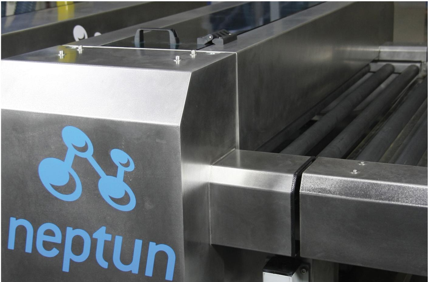
The additional pre-wash module with brushes is complete with upper and lower brush, tank and pump, fan and upper air blade. Particularly suitable for very dirty glass that requires aggressive pre-washing.
