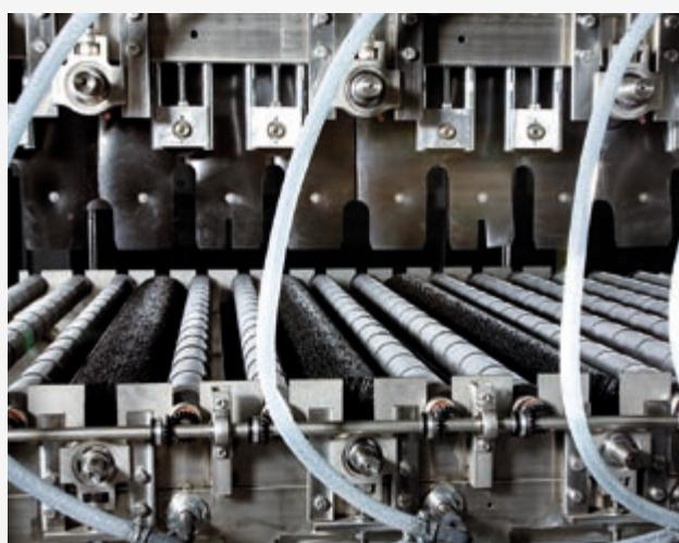
Automatic lifting up system of the upper part up to 500 mm for easy maintenance and inspection.
