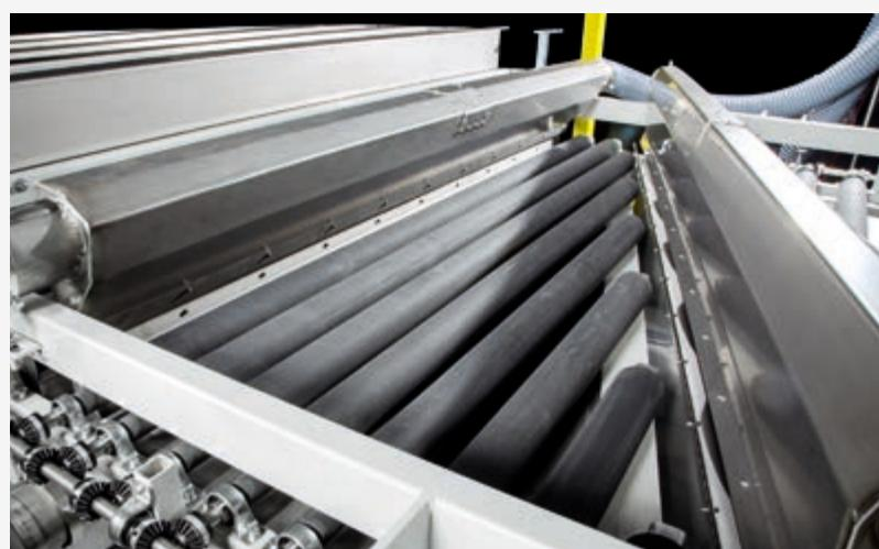
Washing area and drying blades in stainless steel. Air knives and water collecting slide in stainless steel.
