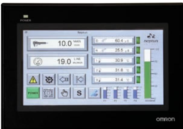
Powerful control unit with touch screen for machine management, fault diagnostics, scheduled maintenance and numerous optional functions:
