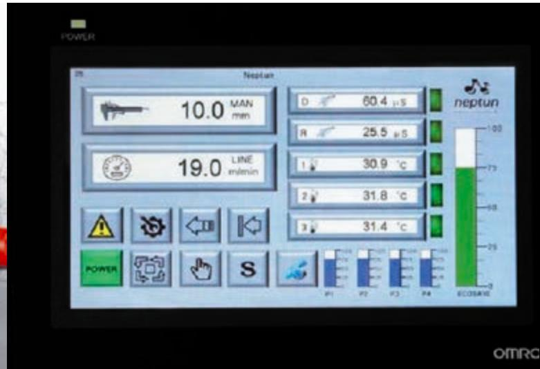
**Wave** is equipped with a powerful control unit with touch screen to manage the machine, remote diagnosis, scheduled maintenance and several innovative functions: water quality control **A-Qual**, energy saving **Ecosave**, **SmartSpeed** for differentiated speed management and optimal drying also of the final glass edge, **NightCare** for pre-heating of the water, programming of the automatic exchange of the water during the night.
