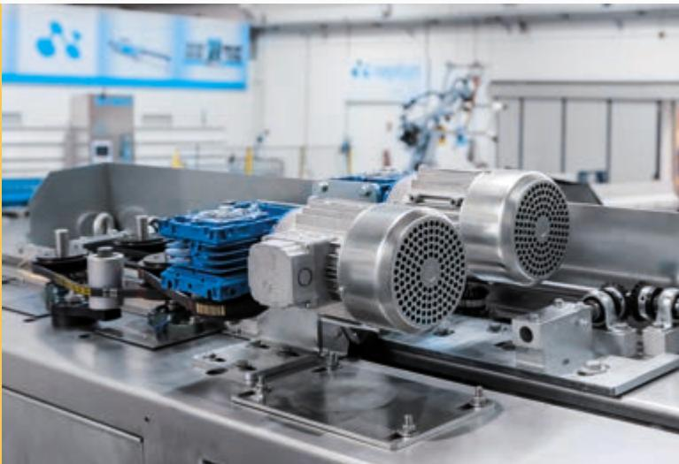
Supporting structure in stainless steel with tempered glass doors, with independent frames for the washing and drying sections. Motorization of front and rear brushes mounted on the structure for better protection from water and humidity.
