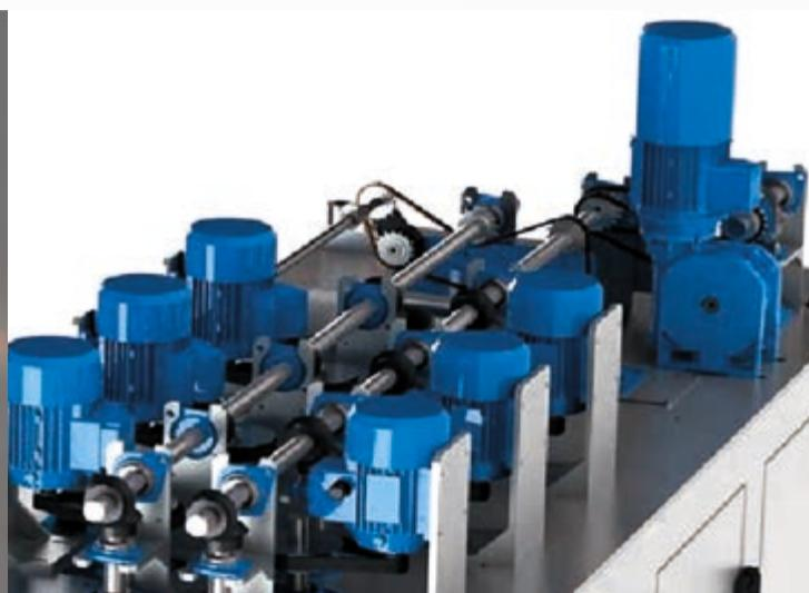
The washing and drying section automatically adapts to the glass thickness up to 60 mm and, upon request, up to 80 mm for an optimal result. Low-E sensor for automatic opening of the first pair of brushes with hard bristle when a low-E glass enters the machine.
