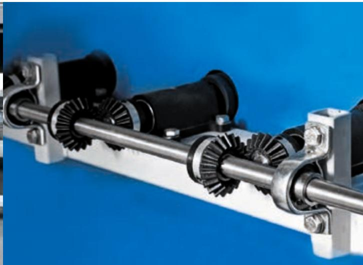
Glass conveying system with rubber scratchproof rollers, driven by maintenance free conical gears. Mechanical transmission in stainless steel. Axes of the conveying rollers and of the brushes made in stainless steel
