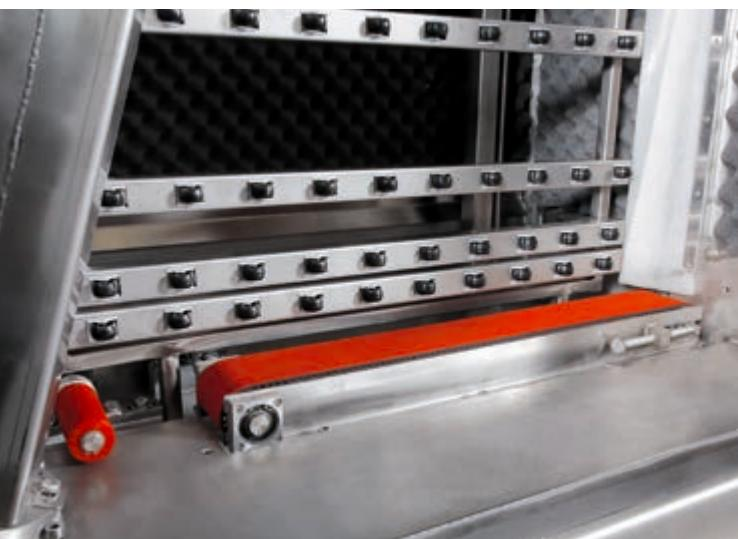
The conveying system in the drying section with touchless belt allows maximum adherence of the edge of the glass and an optimal drying of the surface, without leaving the typical marks of the conveying rollers.
